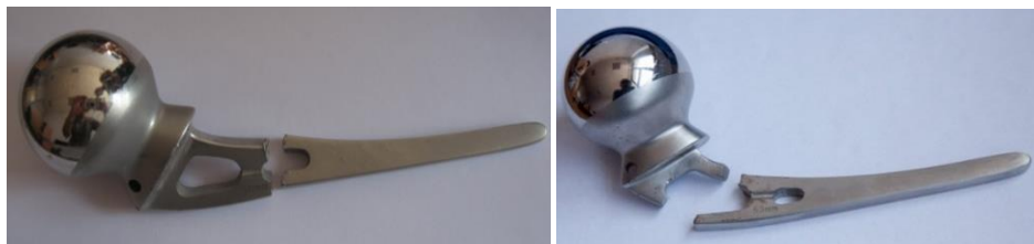
Figure 1. Hip implant fatigue failures
